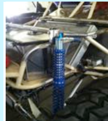
Rattler Gets some Pep in his Step! These pictures show the 2.5 inch KING coil over's that replaced the ORI shocks. The buggy was built as an ultra 4 race buggy. At high speeds the ORI shocks are totally awesome, but were found to be extremely difficult to tune for trails that patrol 3 runs.
